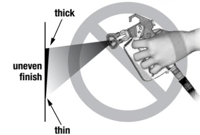
Spray gun tilted downward or upward will produce an uneven finish
