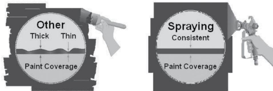
It is important to consider how much faster spraying is compared to other methods. Equally important to your customer is how spraying gives a consistent quality finish, even over rough surfaces.
