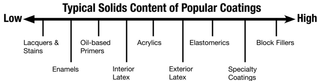
Keeping in mind the typical amount of solids found in coatings (low, medium, or high), allows an easy method for displaying the solids content of popular architectural coatings.
