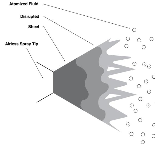
In airless spray, the fast moving high-pressure liquid stream provides the energy necessary to overcome the fluid’s viscosity (resistance to flow) and surface tension (a force that bonds the surface of a liquid together) to form a fine spray.
